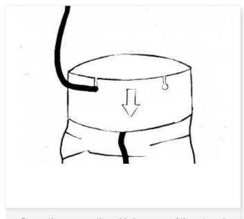
Secure the cover on the cable by means of the external paperboard and the holes made in it.
