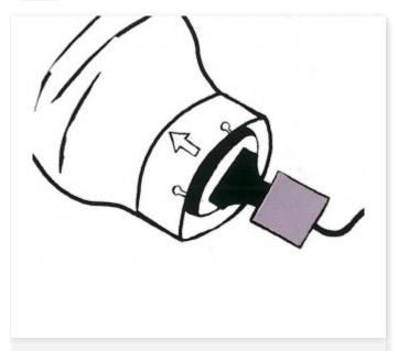
Get the camera head through the paperboard external ring in the arrow-marked direction.
