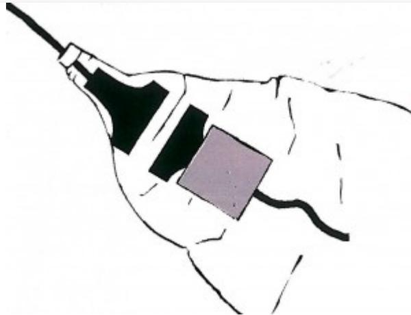
Join the optics with the camera inside the cover.
